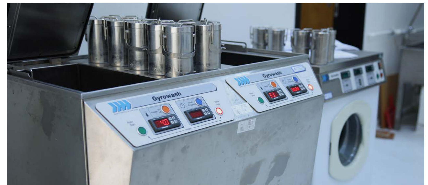
| Gyrowash washing machine washing 4x10 cm sample sizes in accordance with ISO 105-C06 standard
