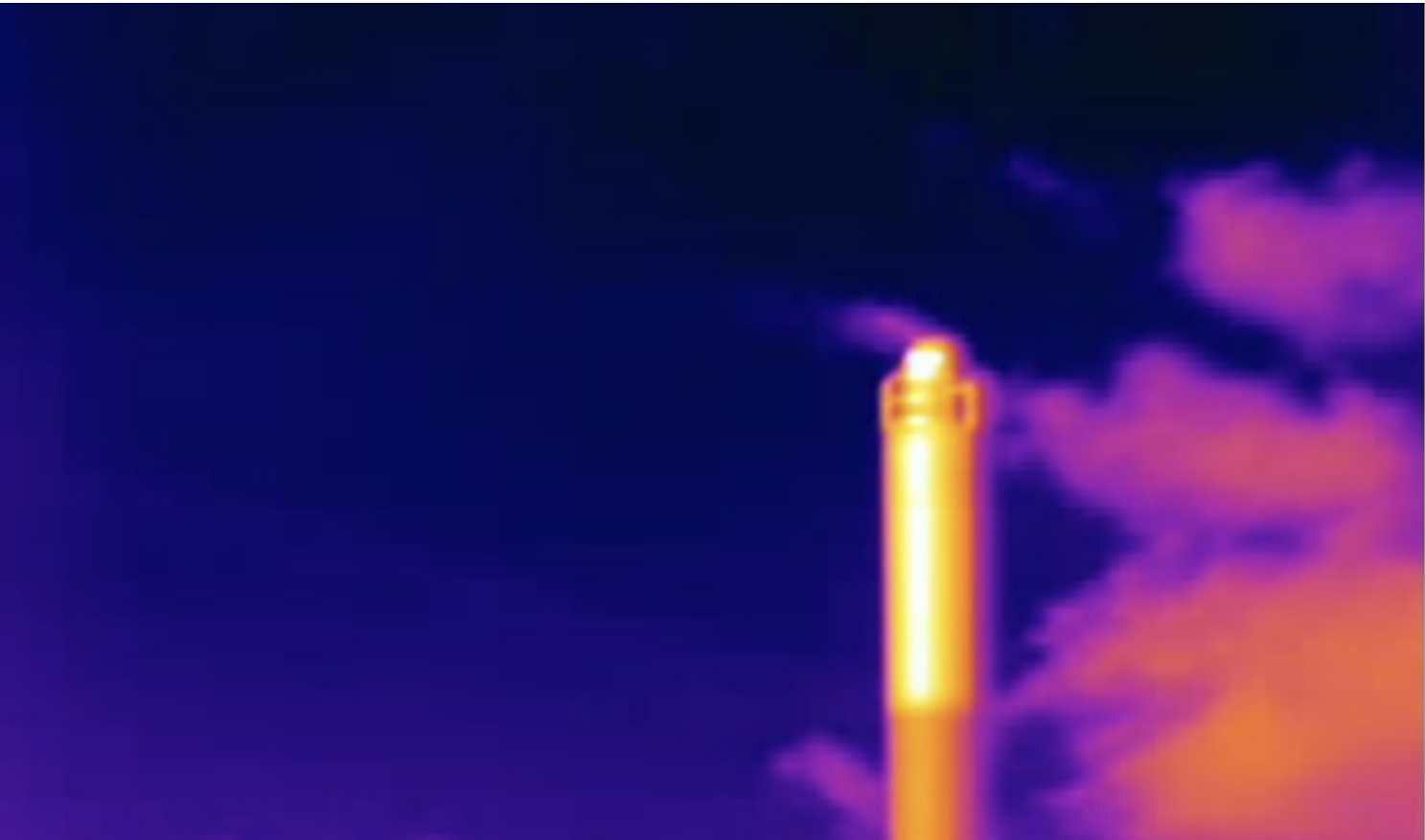
Methane being released through a chimney at Arla's Arinco processing plant
